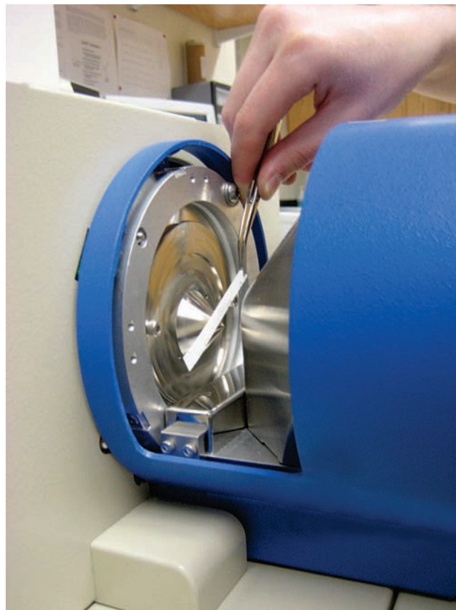
Figure 2. Holding the TLC slide in the DART mass spectrometer. 8
